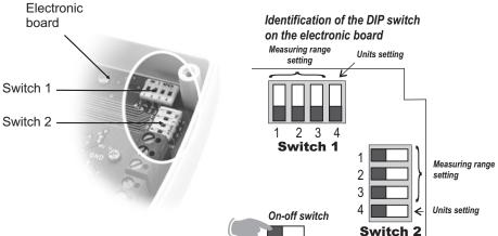
To configure the transmitter, it must not be energized. Then, you can make the settings required, with the DIP switches (as shown on the drawing beside). When the transmitter is configured, you can power it up.
